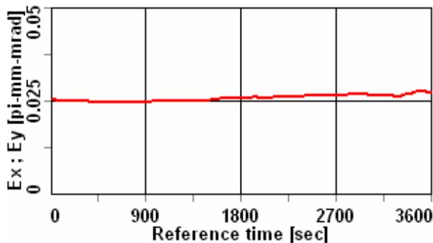
Figure 1: Time evolution of unnormalized transverse rms emittance for typical magnetized cooling parameters of Au ions at 100 GeV/u.
