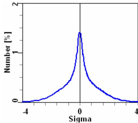
Figure 3: Transverse profile of ion beam after 1 hour of cooling with the “core-tail” IBS approach.
