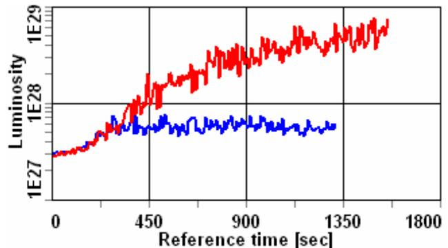
Figure 4: Luminosity growth using IBS approach based the rms of full distribution (red top curve) and using “core-tail” approach (blue), for typical parameters of the magnetized cooling for Au ions at 100 GeV/u.
