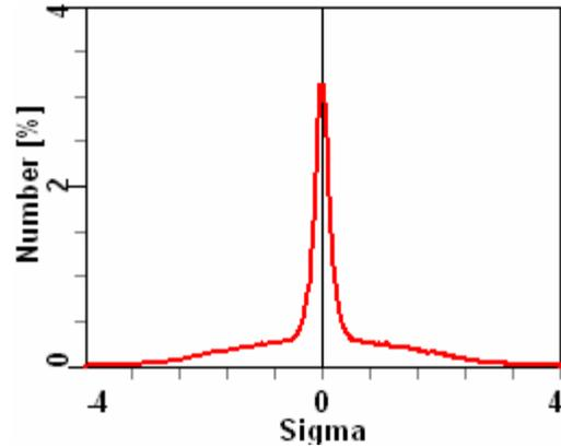
Figure 2: Transverse profile of ion beam after 1 hour of cooling with the IBS calculation based on rms values of full distribution.
