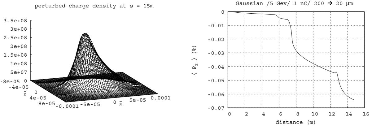
Figure 2: Left: Perturbed charge density at  $s = 15m$  (end of chicane). Right: Mean of the relative energy loss.
