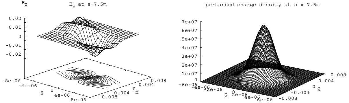
Figure 1: Left:  $E_z$  at  $s = 7.5m$  (end of 3<sup>rd</sup> magnet of the chicane). Right: Perturbed charge density at  $s = 7.5m$ .
