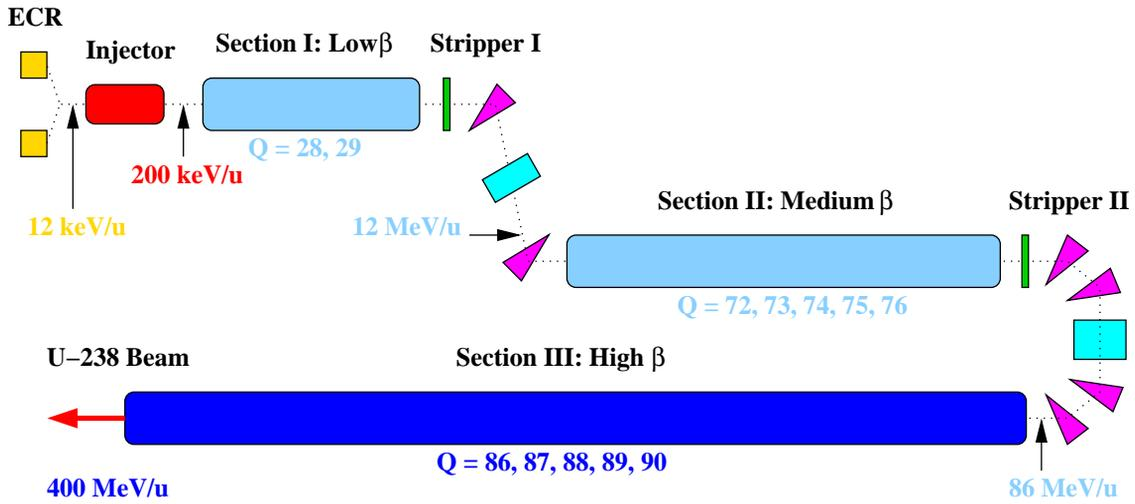
Figure 1: Schematic of the RIA driver linac.
