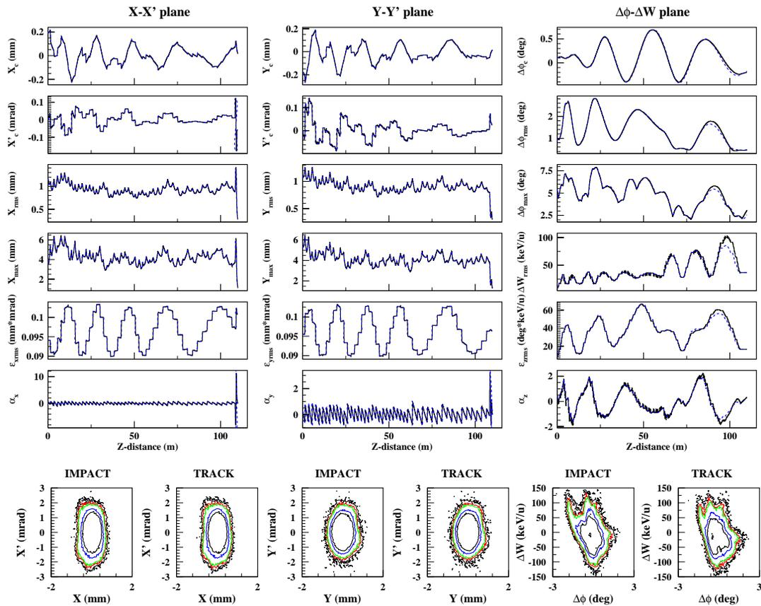
Figure 3: Comparison of IMPACT and TRACK simulations of the second linac section for a five charge state uranium beam ( $Q=72,73,74,75,76$ ). The black solid curves corresponds to IMPACT and the blue dashed curves to TRACK, see Fig. 2 for more details.
