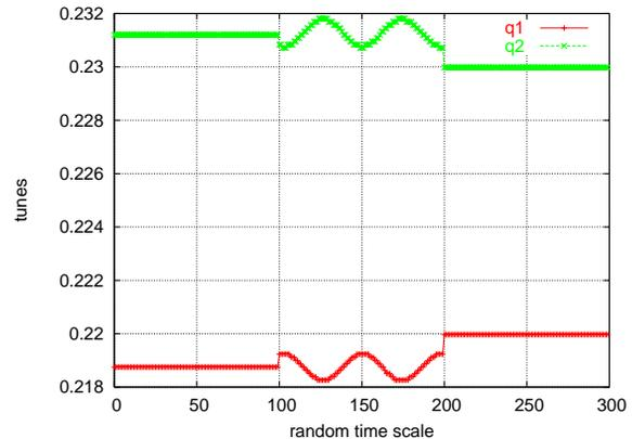
Figure 3: The tunes in the whole procedure of global decoupling in the simulation.
