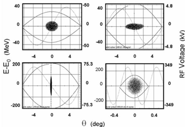
Figure 1: Phase space ( $\Delta E$ ,  $\theta$ ) distributions from 8 to 150 GeV. First plot is 2.5 MHz bunch at injection. Second plot is the end of first rotation at 27 GeV at minimum bunch height. Third plot is the end of second rotation at 27 GeV at minimum bunch width. Fourth plot is the 53 MHz bunch at 150 GeV.
