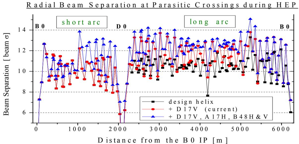
Figure 1: Separation between protons and antiprotons at all parasitic crossings for the design separator configuration (black squares), with the addition of vertical separators at the D17 location (red circles), and with all proposed additional separators (blue triangles).
