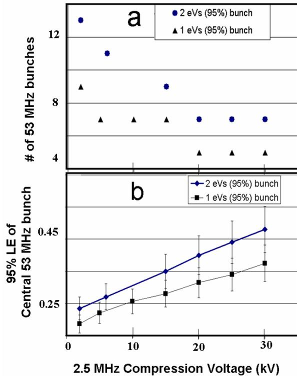
Fig.1. ESME simulations for 8 GeV bunch compression of 2.5 MHz pbar bunches in the MI. a) Number of 53 MHz bunches vs compression voltage and b) 53 MHz LE vs compression voltage.
