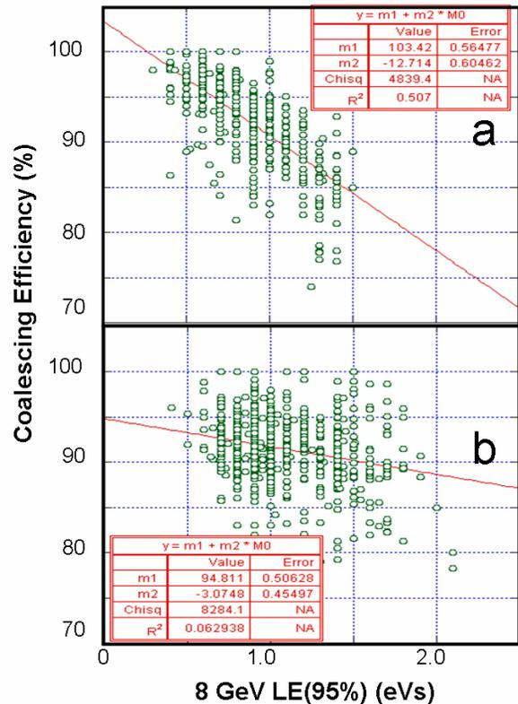
Figure 2: Measured pbar coalescing efficiency at 150 GeV in the MI as a function of 8 GeV LE. a) Before and b) after implementation of the new scheme. This data is from Accumulator transfers.
