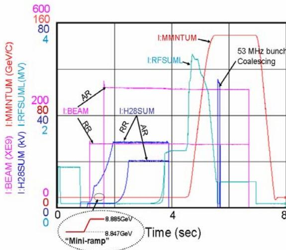
Figure 4: Experimental data on pbar injection, rf manipulations, acceleration and coalescing. I:BEAM, I:H28SUM, I:MMNTUM and I:RFSUML measure beam current, 2.5 MHz rf voltage, magnet ramp and 53 MHz rf voltage, respectively. The Mimi-Ramp is also shown.
