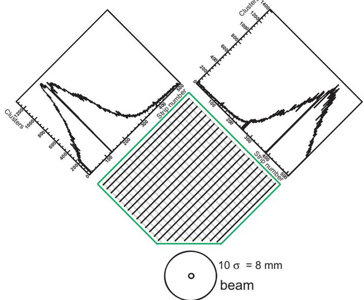
Figure 3: Profile of the beam halo as seen by two detector planes with orthogonal strip orientations at a distance of 10 mm from the beam centre.
