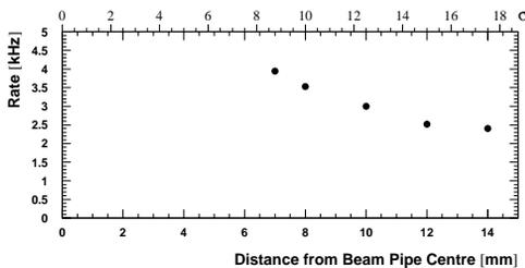
Figure 2: Trigger rate as a function of the window's distance from the beam pipe centre.
