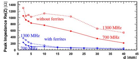
Figure 8: Impedance as a function of  $d$  at the two dominant resonances.
