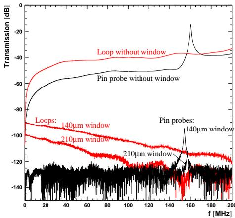
Figure 5: Signal transmission from the wire to the antennas as a function of the frequency for a distance of 2 mm between each pot and the wire in the centre. The peaks at 160 MHz are caused by a resonance of the pin probe. Corrections for reflections at Port A and for the 30 dB amplification have been applied.
