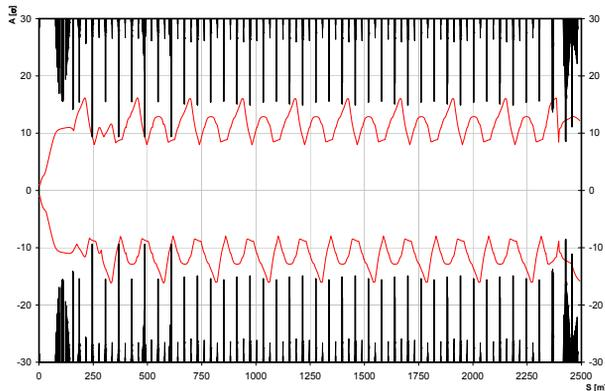
Figure 6: Expected and measured horizontal aperture in TI 8, for nominal beam optics. The measured aperture is about 8.2 nominal  $\sigma$ .
