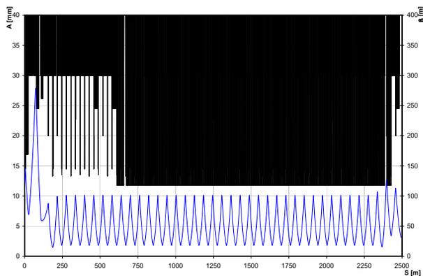
Figure 2: Vertical physical aperture model for TI 8, together with the vertical beta function.
