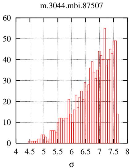
Figure 5: Monte-Carlo results (counts per 0.1  $\sigma$  bin) showing the distribution of aperture limits for 1000 simulated TI 8 states with all errors.
