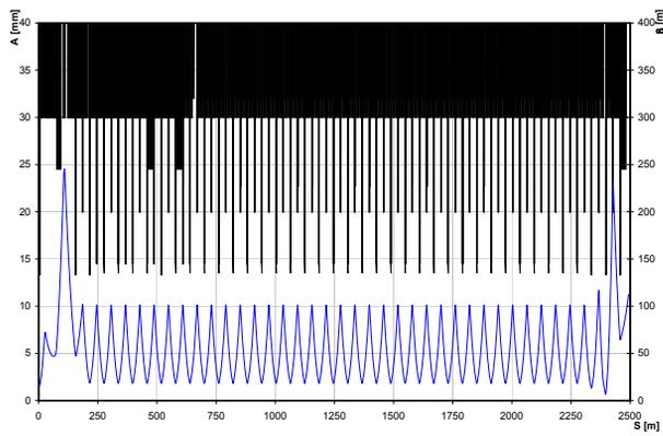
Figure 1: Horizontal physical aperture model for TI 8, together with the horizontal beta function.
