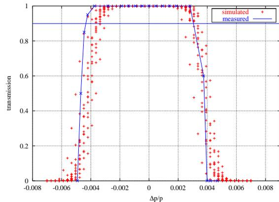
Figure 7: Simulated and measured transmission of TI 8, for different beam energy offsets, for nominal beam optics.
