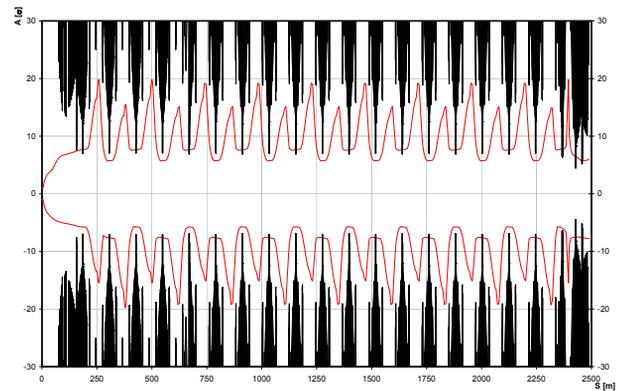
Figure 3: Expected and measured horizontal aperture in TI 8, for the perturbed beam optics. The measured aperture is about 5.8 nominal  $\sigma$ .
