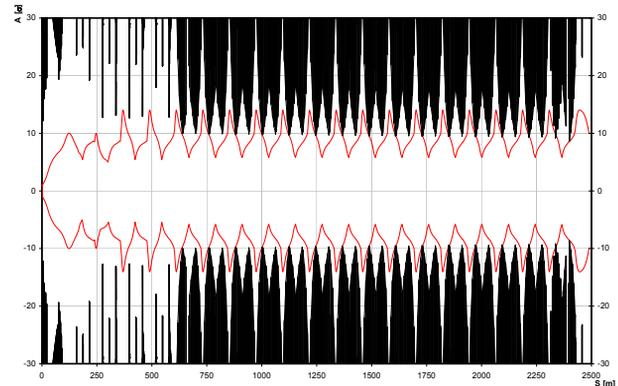
Figure 4: Expected and measured vertical aperture in TI 8, for the perturbed beam optics. The measured edge of the beam envelope (red) is compared to the calculated aperture (black). The measured aperture is about 5.1 nominal  $\sigma$ .
