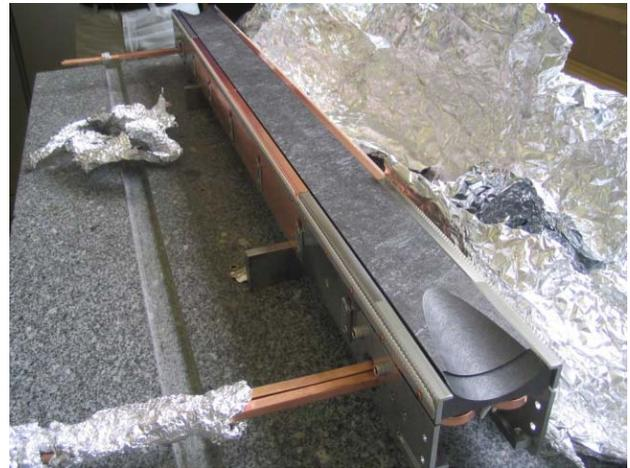
Figure 1: Secondary LHC collimator jaw. The 1 m long flat carbon surface and tapering at both ends, the support and Cu cooling is visible.
