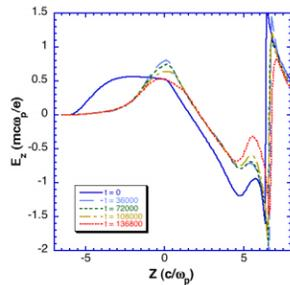
Figure 2: Longitudinal wakefield evolution for the 100 GeV simulation.
