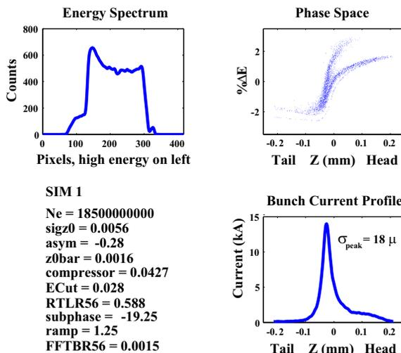
Figure 3: Simulation output showing bunch phase space.
