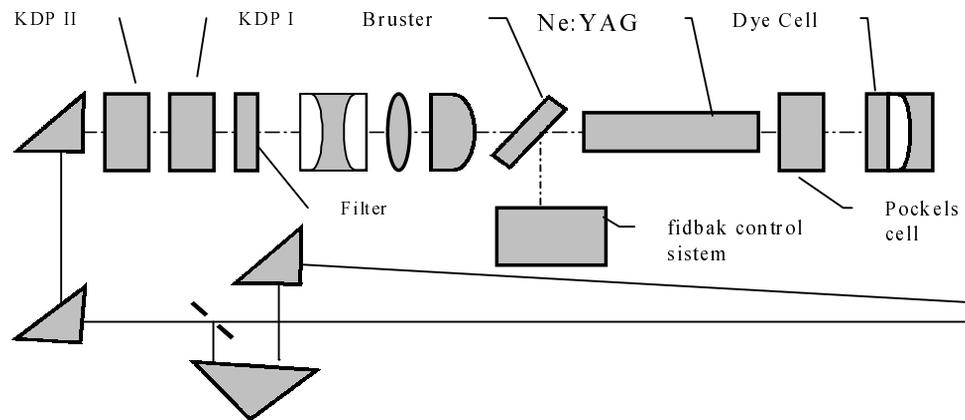
Figure 2: The scheme of laser set-up.
