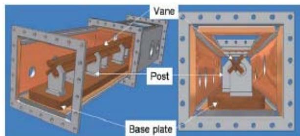
Figure 3: The lateral and cross-sectional view of RFQ.
