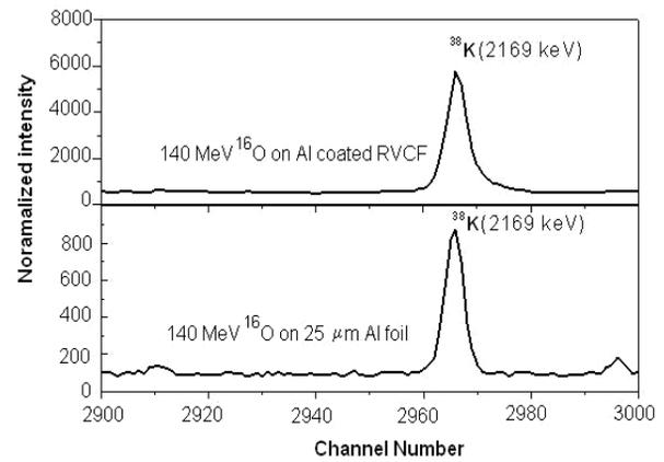
Figure 2: The normalized intensity of 2169 keV gamma ray from the decay of  $^{38}\text{K}$  produced from “thick” and “thin” aluminum targets.
