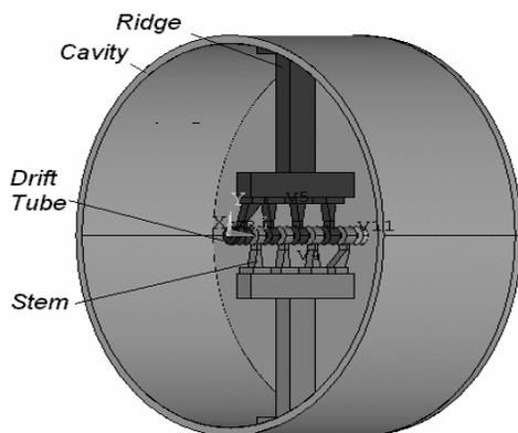
Figure 4: Schematic diagram of IH-Linac Tank.
