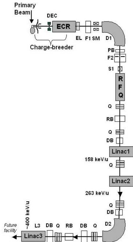
Figure 1: Layout of VEC-RIB Facility.
