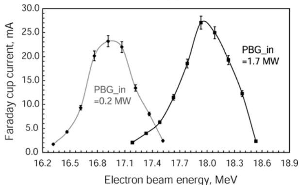
Figure 4: The Faraday cup signal at the 30-degree-bend spectrometer arm versus the electron beam energy for different input powers into the PBG accelerator.
