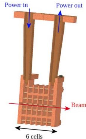
Figure 1: Cut away drawing of a six-cell PBG accelerator.
