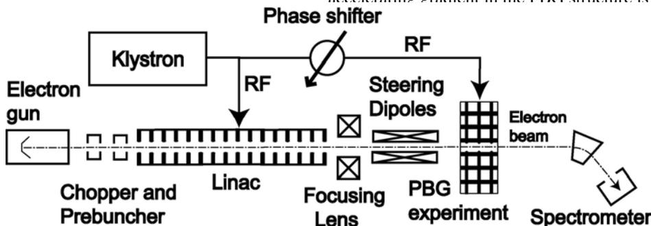
Figure 3: The hot test experimental setup schematics.
