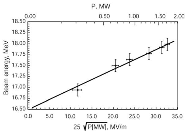
Figure 5: Measured energy of the electron beam versus square root of the PBG accelerator input power,  $P$ .
