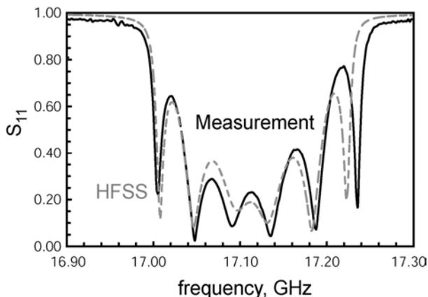
Figure 2: Comparison between the computed and measured  $S_{11}$  coupling curves for the 6-cell PBG accelerator structure.
