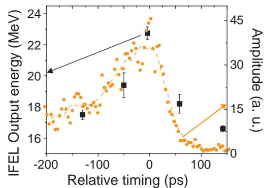
Figure 2: IFEL output energy vs. measured delay on the streak camera between reference e-beam pulse and CO<sub>2</sub> laser. Also shown is a typical streak of the CO<sub>2</sub> laser pulse.
