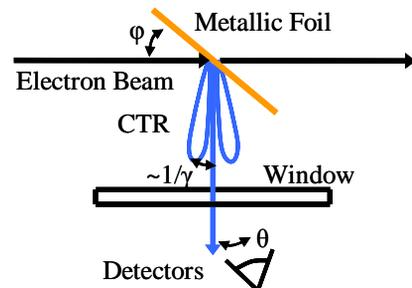
Figure 1: Schematic of experimental setup,  $\phi$  is the orientation angle of the foil with respect to the beam,  $\theta$  is the observation angle.
