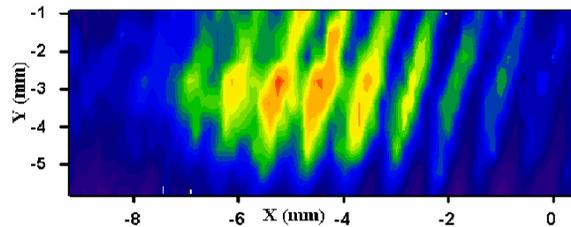
Figure 5: Measured dependence of the radiation yield as a function of the vertical target position.
