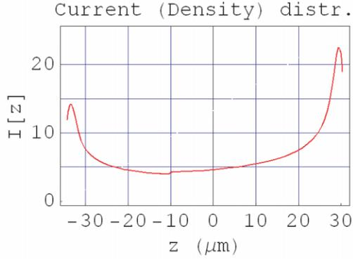
Figure 2: Bunch longitudinal distribution after BC2.
