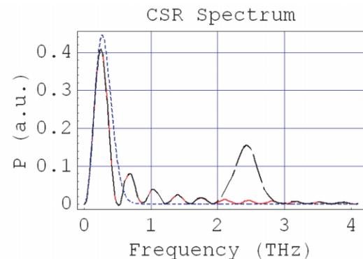
Figure 7: CSR spectrum with 5-% amplitude modulation after BC1. The long-dashed curve (black) is for the parabolic distribution with 5-% modulation; the solid (red) is for the parabolic distribution without modulation; the dashed (blue) is for a Gaussian.
