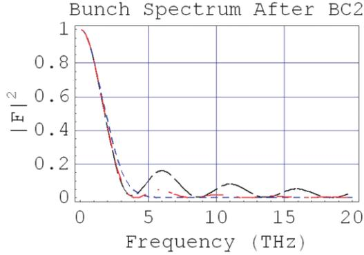
Figure 3: Bunch spectrum after BC2. Long dashed curve (black) is for the double-horn distribution; dashed curve (blue) is for a Gaussian distribution, and dash-dotted (red) is for a step function.
