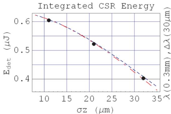
Figure 5: Detected CSR energy as a function of bunch length. The dot (black) is for the double-horn distribution, and the curves have the same meaning as in Fig. 3.
