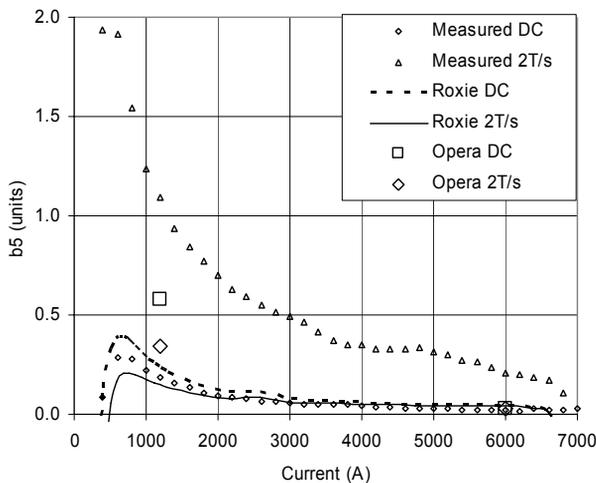
Figure 6: Decapole term coming from the superconductor (in units of  $10^{-4}$  @ 25 mm radius).
