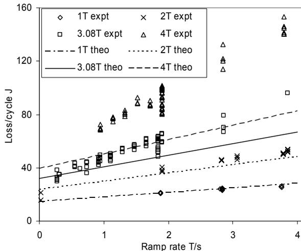
Figure 3: Losses per cycle versus dB/dt.
