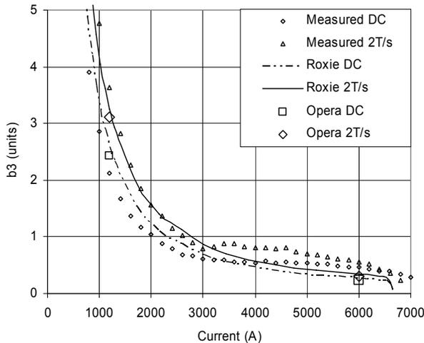
Figure 5: Sextupole term coming from the superconductor (in units of  $10^{-4}$  @ 25 mm radius).
