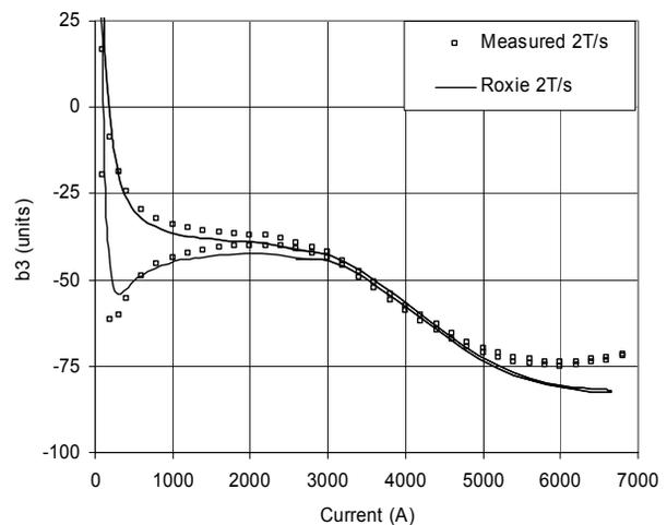
Figure 4: Measured sextupole field (in units of  $10^{-4}$  @ 25 mm radius).
