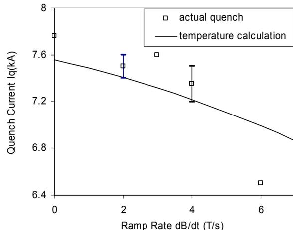
Figure 2: GSI 001 quench current  $I_q$  versus ramp rate dB/dt.
