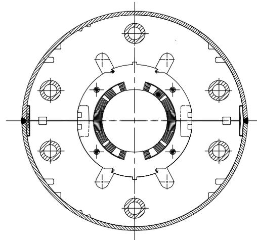
Figure 1: Cross section of the magnet.
