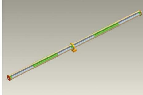
The RTBT dipole will be mapped using the above rotating “Halbach” style planer coil. At the moment, this coil is being assembled her at SNS. The magnet will be mapped in-situ using the installed power supply.
