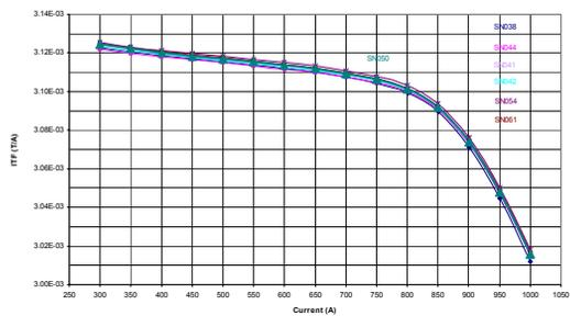
In the RTBT there will be three sets of four Quads and one set of three Quads. Each set will be on a common power supply. The Quads within each set have to be matched within 0.1%. In the above data, there are one set of four and one set of three matched to 0.1%.
