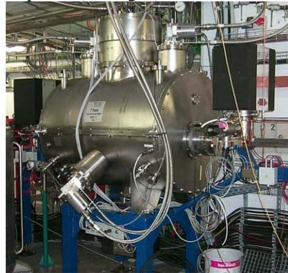
Figure 5: Photo of the 7 Tesla 3-pole WLS for BESSY-2.
