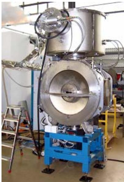
Figure 15 Assembled BESSY-2 Superbend.
