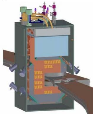
Figure 13 Schematics of an ALS Superbend magnet.
