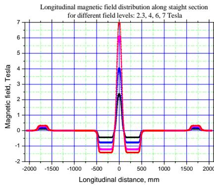
Figure 3: Magnetic field distribution of the 7 Tesla WLS for BESSY-2.
