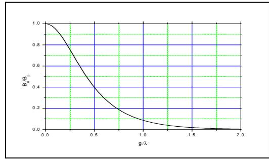
Figure 9: Behaviour of peak field in median plane vs. the ratio  $g/\lambda$  for the same type of superconducting wire.
