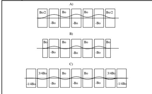
Figure 6: Orbit distortion inside wigglers with different magnetic structures.
