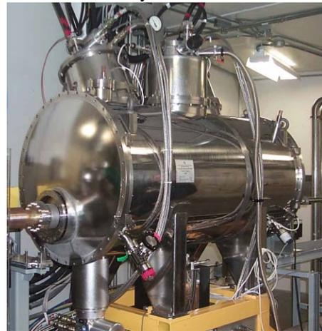
Figure 10 2 Tesla 63-pole superconducting wiggler with zero liquid helium boil off for Canadian Light Source.
