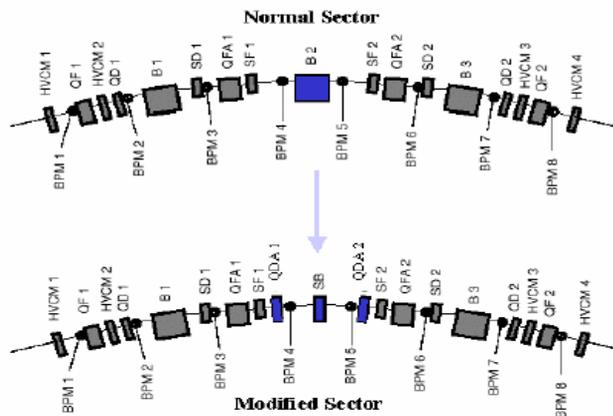
Figure 12 Magnetic layout of a normal (top) and modified (bottom) sector.
