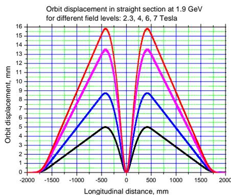
Figure 4: Orbit distortion inside the 7 Tesla SC WLS for BESSY-2.
