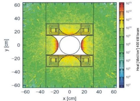
Figure 3: Simulation of heat deposition in the first quadrupole of the pre-separator, for a 500 MeV/u  $^{48}\text{Ca}$  primary beam.
