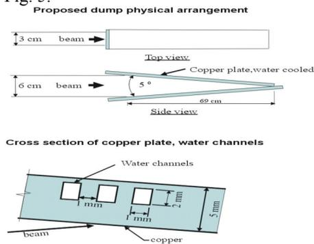
Figure 5: Water-cooled copper stationary beam dump concept.
