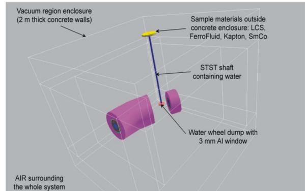
Figure 6: Geometry for a rotating water-cooled aluminum wheel dump concept used in simulations.
