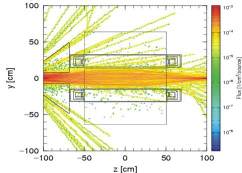
Figure 4: Simulation of the pre-separator first quadrupole using PHITS. Levels of proton flux are shown, for a  $^{48}\text{Ca}$  beam at 500 MeV/u. The magnetic field option was used.
