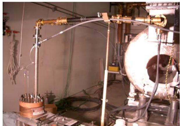
Figure 2. Muons Inc. rf cavity and SC solenoid in MTA.
