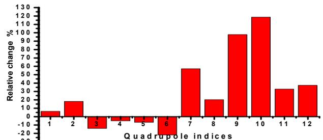
Figure 4: Relative change of quadrupole strength in the new compensation scheme obtained by MAD-X.
