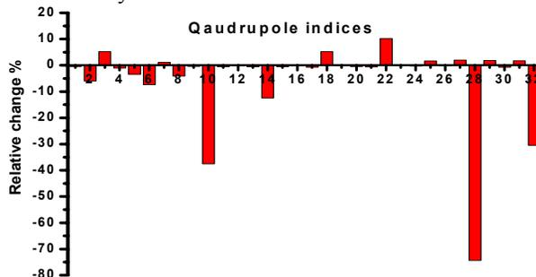
Figure 6: Relative change of quadrupole strength in the new compensation scheme obtained by LOCO code.
