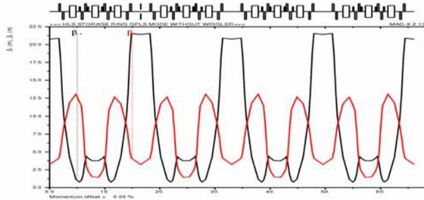
Figure 1: Beta-functions of HLS storage ring without wiggler.
