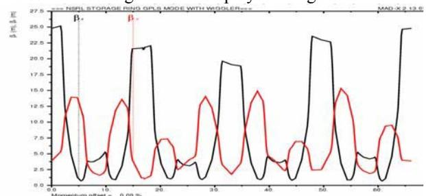
Figure 3: Beta-functions of the new compensation scheme obtained by MAD-X.
