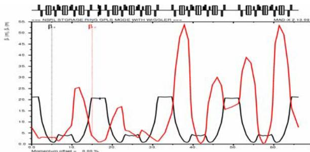
Figure 2: Beta-functions of the tune compensation scheme for HLS storage ring.
