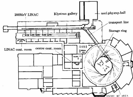
Figure 1: Layout of HLS and its 200MeV linac injector.
