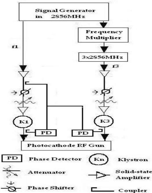
Figure 4: Configuration of RF system for a two frequency RF photocathode gun.
