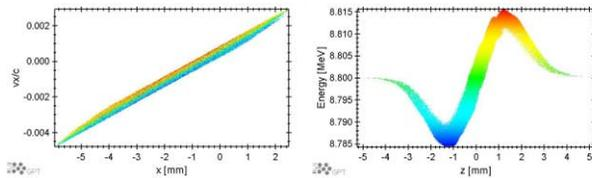
Figure 5: Transverse and longitudinal distribution at the end of the injector line of ERLP.
