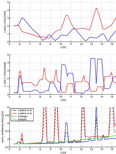
Figure 4: Transverse beam sizes, divergences and normalized emittance for a Gaussian distribution with space charge for GPT, together with the analytic estimate, for the injector model including dipoles.
