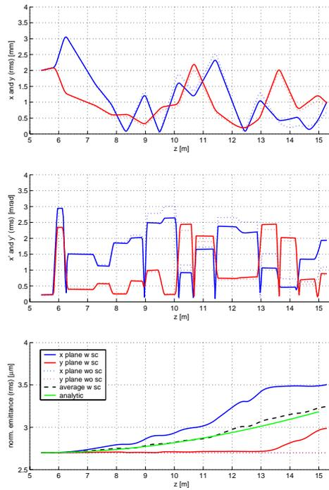
Figure 2: Transverse beam sizes, divergences and normalized emittance for a Gaussian distribution with space charge using ASTRA, together with the analytic estimate, for the axially-symmetric model.
