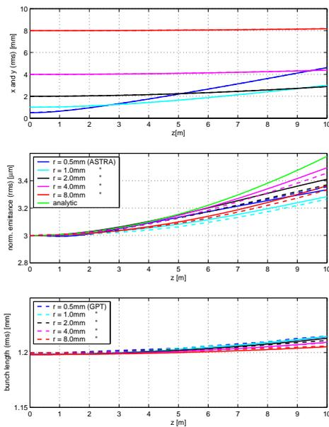
Figure 1: RMS beam size ( $2r$  in plot), normalized emittance and bunch length increase for  $\epsilon_{n0} = 3 \mu\text{m}$ .
