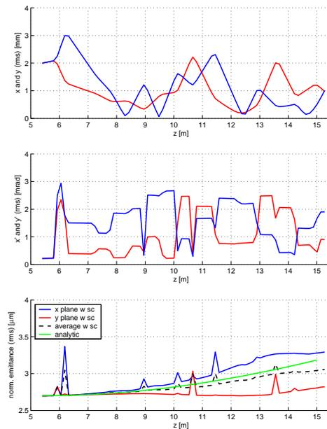
Figure 3: Transverse beam sizes, divergences and normalized emittance for a Gaussian distribution with space charge using GPT, together with the analytic estimate, for the axially-symmetric model.
