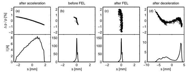
Figure 3: Longitudinal phase space and bunch profile at different locations in the ERLP: (a) after off-crest acceleration by  $\varphi_{rf} = 7.8^\circ$ ; (b) after the compressor chicane with the sextupoles set to  $100 \text{ m}^{-3}$ ; (c) after FEL interaction; (d) after energy recovery.
