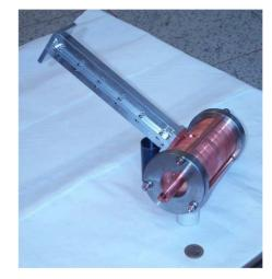
Figure 4: copper prototype of the X band structure.
