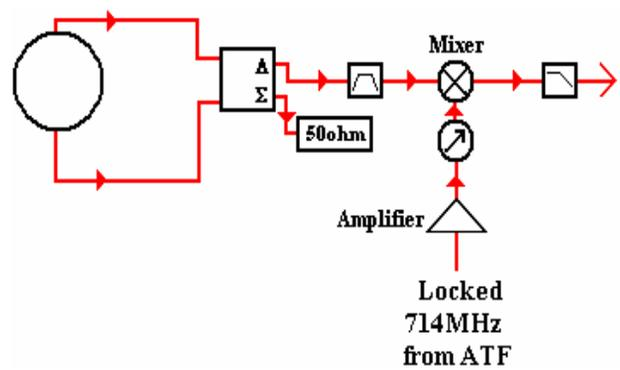
Figure 4: Schematic of BPM signal processor.
