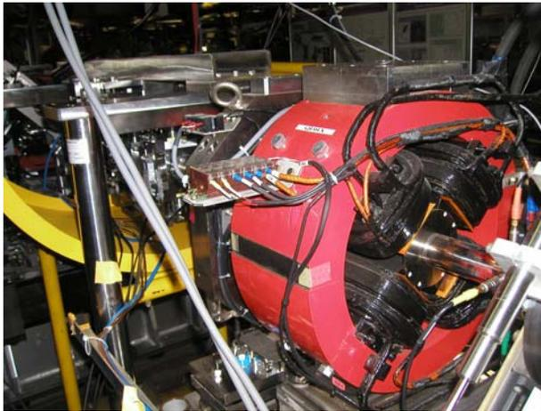
Figure 3: ATF beamline showing the kicker (left) and BPM (right).
