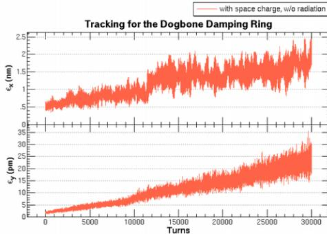
Figure 1: The horizontal(upper) and the vertical(lower) emittance growth due to the space charge effect. The synchrotron radiation is turned off. The emittances increase almost linear in time. It will be safe if the growth rate is much smaller than the synchrotron radiation excitation.
