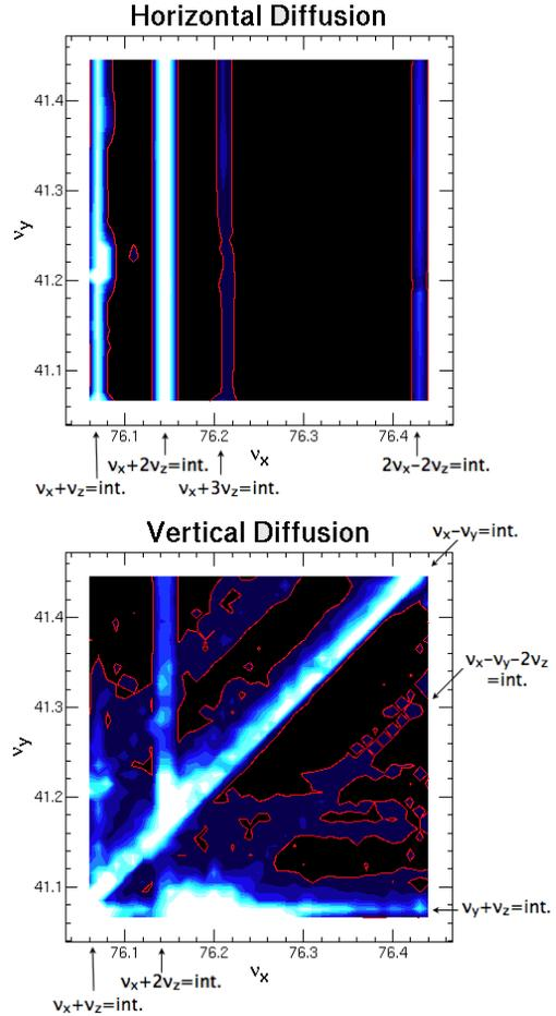
Figure 2: The tune space of the horizontal(upper) and vertical(lower) emittance diffusion rate due to the space charge effect. Darker area has smaller diffusion rate, and the red line shows 1/5 of the synchrotron radiation excitation. Several resonance lines are seen.
