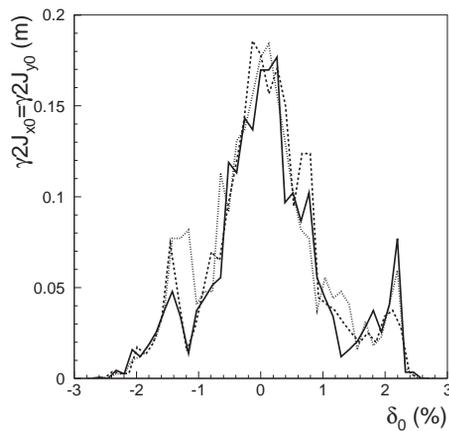
Figure 3: Comparison of the dynamic aperture including the wiggler nonlinearity and the space charge effect (solid), the wiggler nonlinearity without the space charge (dotted), and without both (dashed).
