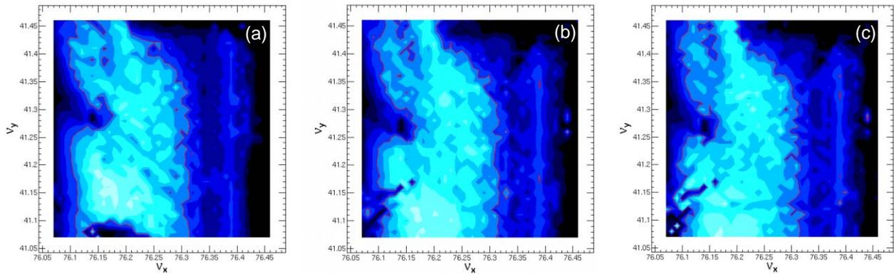
Figure 4: Tune survey of the dynamic aperture: (a) without wiggler nonlinearity and space charge, (b) with wiggler nonlinearity, without space charge, (c) with wiggler nonlinearity and space charge. The red lines show acceptable regions.
