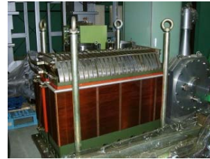
Figure 3: Pulse-transformer of JHP is modified for STF. waveform shows the forward travelling wave.
