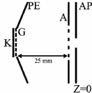
Figure 1: A highly simplified schematic (not to scale) of the UMER electron gun: cathode (K), control grid (G), Pierce electrode (PE), anode (A), and aperture plate (AP)
