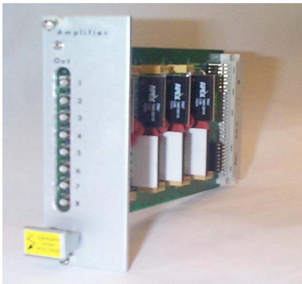
Figure 3: Deflection plates high-voltage amplifier.
