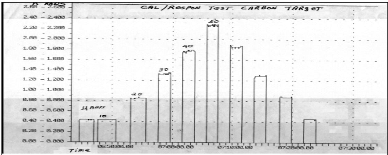
Figure 5: Calibration Testing of System. Radiation levels produced by each target, energy and current can be graphed and archived to assist in selecting trip points levels for a given experiment and hall conditions.
