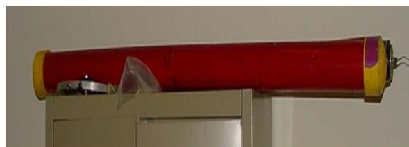
Figure 1C: 10-Foot Ion Chamber in ABS Housing.
