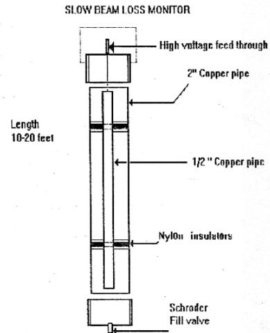
Figure 1A: Schematic Layout of Probe.
