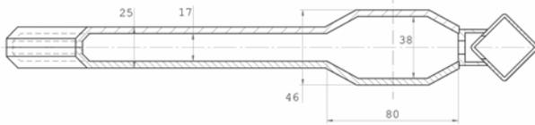
Figure 4: Cross section of steel chamber in new octant. The NEG pumping channel is located on the right side.
