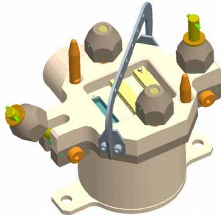
Figure 10: RH HARP and signal and control cable connector.
