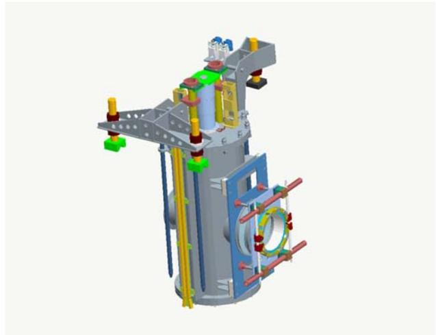
Figure 5: HARP vessel assembly.
