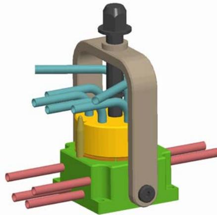
Figure 11: RH HARP six-way air control connector.
