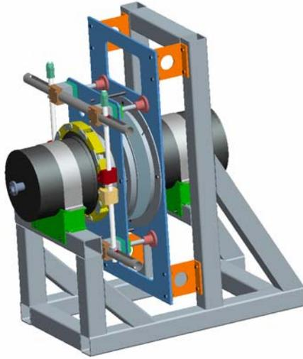
Figure 7: RH vacuum connection and clamp test rig.
