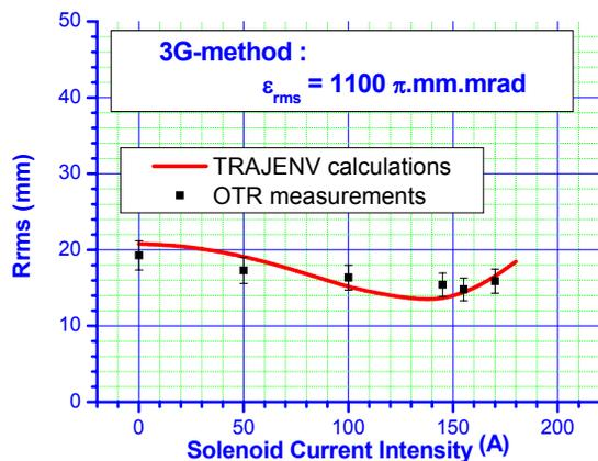
Figure 5: Beam radius evolution as a function of the current intensity drawn into the second focusing coil with respect to figure 1.
