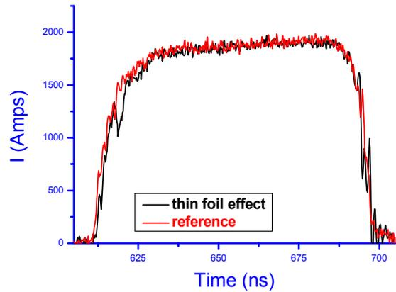
Figure 3: First BPM signal downstream the foil for a beam shot with the foil put into (black curve) or removed from (red curve) the line.
