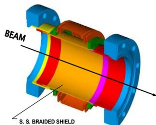
Figure 2: Shielded Bellows.
