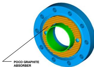
Figure 3: Zero Length Beam Clipper.
