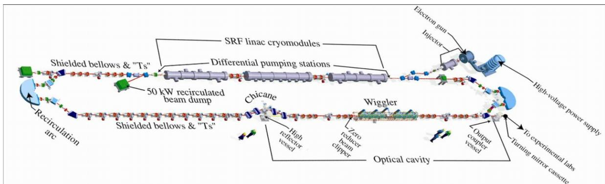
Figure 1: 10kW IR FEL Machine and Component Locations.
