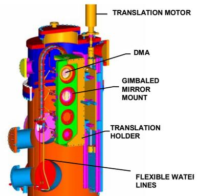
Figure 6: Optical Cavity High Reflector Vessel.
