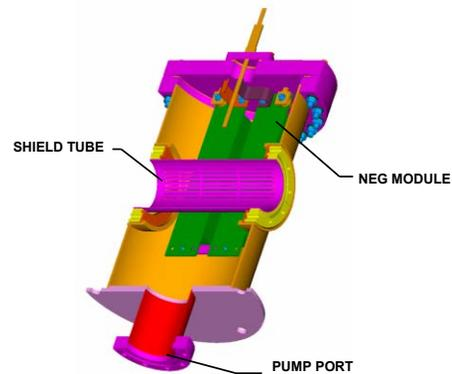
Figure 4: Differential Pumping Station.
