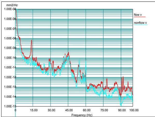
Figure 4. Compare the water flow and no flow on the Q magnet vibration in the vertical direction.
