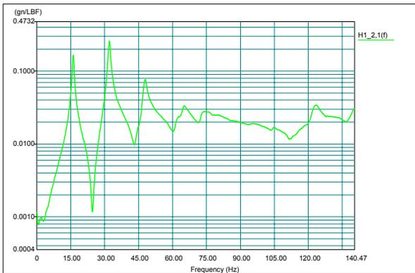
Figure 1: Frequency response function of magnet girder.
