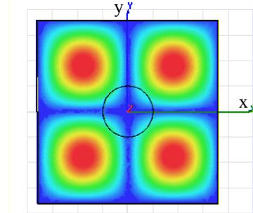
Figure 1: Field pattern in a rectangular cavity with a beam pipe. Shading indicates  $|E_z|$  on the midplane, and the circle is the beam pipe.
