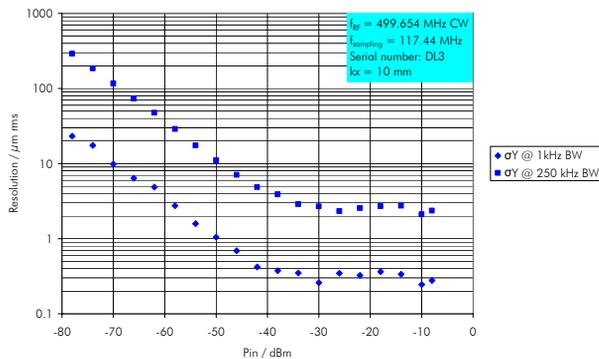
Figure 7: Resolution at two different bandwidths.
