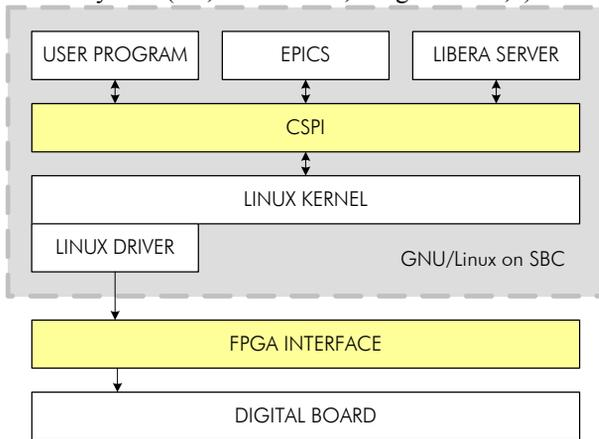
Figure 6: Software Architecture.
