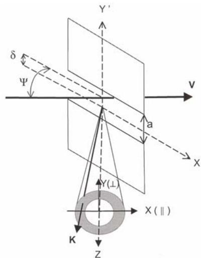
Figure 2: A schematic of the generation of ODR by a charged particle beam as it passes near a metal plane (based on Fig. 1 of reference 4.)
