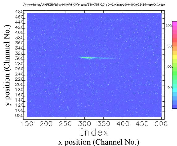
Figure 4: The observed ODR "image" of the 7-GeV beam with  $Q = 3.3$  nC and  $d = 2.00$  mm.
