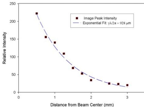
Figure 6: A plot of the experimental dependence of the signal peak intensity versus the blade edge position.
