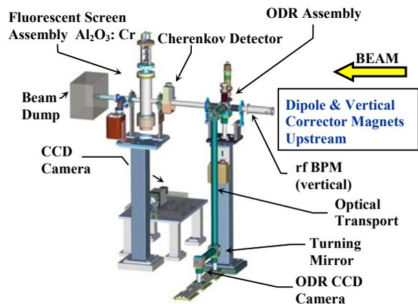
Figure 1: A schematic drawing of the rf BPM, ODR assembly, Cherenkov detector, beam profile screen, and beam dump. The optical transport to the CCD camera is also indicated.
