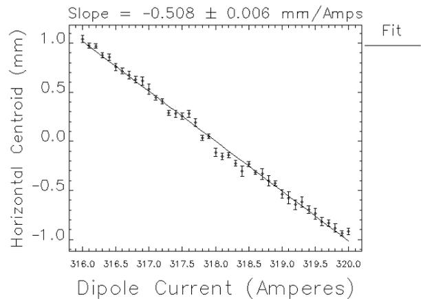
Figure 7: A plot of the ODR horizontal image centroid versus the dipole magnet current supply set point. A  $50\text{-}\mu\text{m}$  relative position sensitivity is observed.
