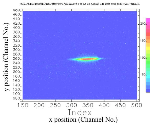
Figure 3: The observed OTR image of the 7-GeV beam with  $Q = 0.4$  nC.
