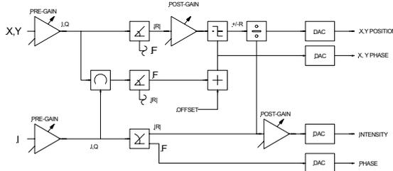
Figure 4: Firmware functional block diagram.
