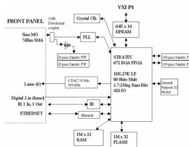
Figure 3: Motherboard components.
