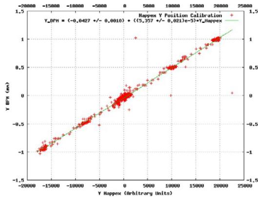
Figure 5: Calibration of the HAPPEX Y measurement against an existing BPM.
