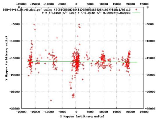
Figure 8: The X position was varied by  $\pm 2$ mm and no change observed on the Y position.
