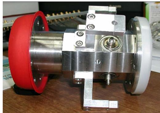
Figure 2: Fabricated strip-line BPM.
