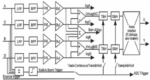
Figure 5: Log-ratio BPM block diagram.
