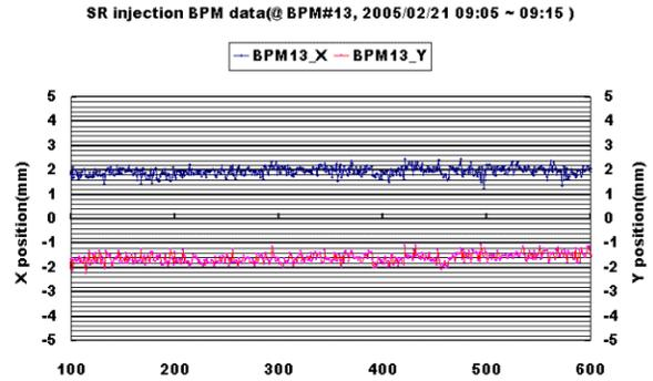
Figure 8: BPM data of BPM#13 at 2005/02/21 09:00 SR injection time.
