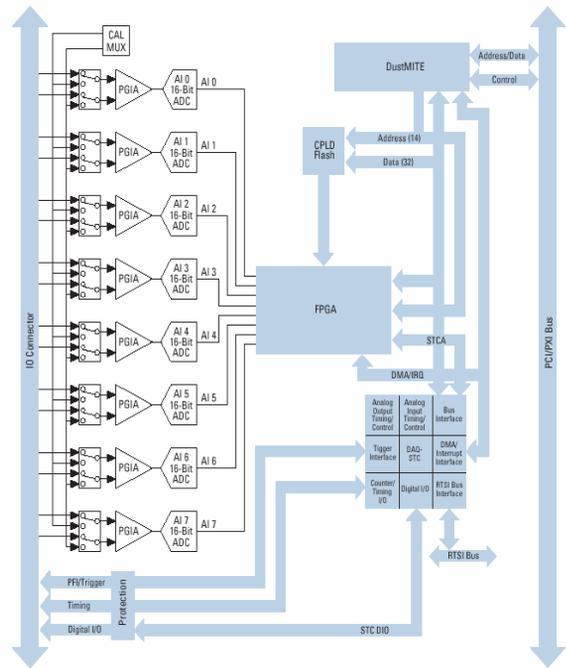
Figure 6: Block diagram of NI 6143 DAQ board.
