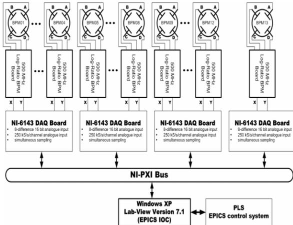
Figure 7: Block diagram of BTL BPM data acquisition system.
