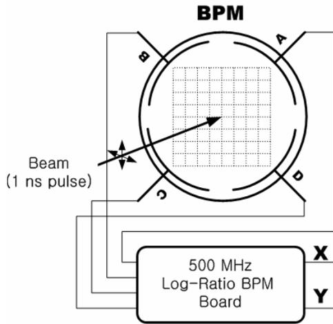
Figure 3: BPM test set-up.
