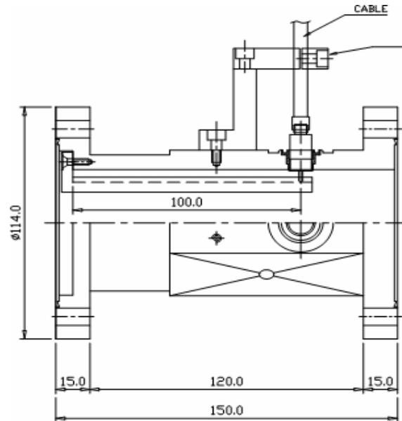
Figure 1: The strip-line type BPM for PLS BTL.
