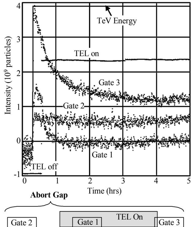
Figure 4: Typical abort gap beam intensity behavior at the beginning of a store. No signal is present until the beam energy is at its operating level of 980 GeV. The TEL turns on ~15 minutes later. At that time, gate 1, which overlaps the TEL, is cleaned out. The beam that is in the abort gap when the energy reaches 980 GeV is a captured remnant left over from coalescing. The bottom diagram shows the relative timing of the gates and the TEL.
