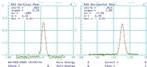
Figure 1: The ACNET program display for the Flying wire measurements of an antiproton beam.
