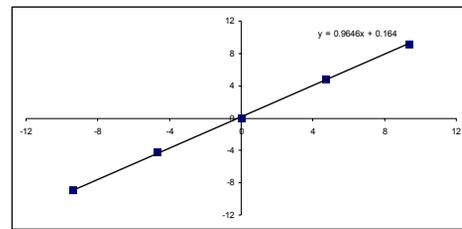
Figure 2: Peak position measured with the horizontal Flying wire vs. calculated three-bump displacement. The slope from the linear fit is 0.965. The data is similar for the vertical.
