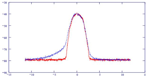
Figure 3: The measured energy spectra of the beam before (red trace) and after 20 wire crossings of the beam (blue trace). The vertical axis is on logarithmic scale. The horizontal unit is in MeV. The computed total ionization energy loss based on the analysis of the Landau distribution is  $0.088 \pm 0.004$  MeV.
