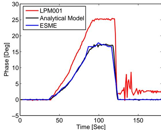
Figure 3: Comparison between the longitudinal phase monitor (LPM001), an analytical model and ESME during the ramp of store #4121.
