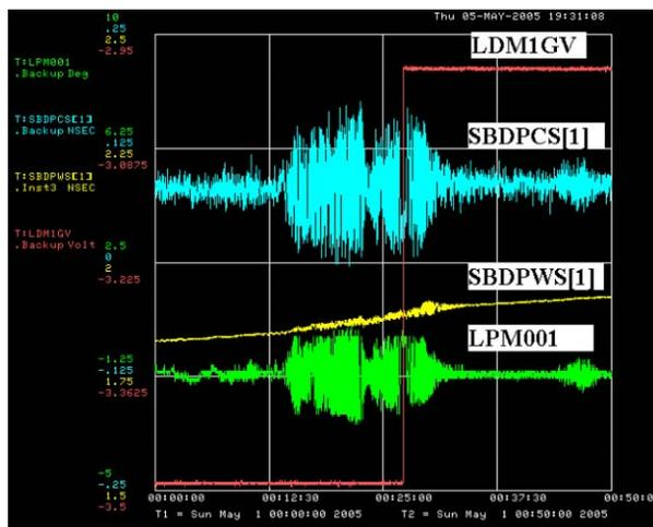
Figure 5: Longitudinal instabilities of the first proton bunch reported by the longitudinal phase monitor (store # 4121).
