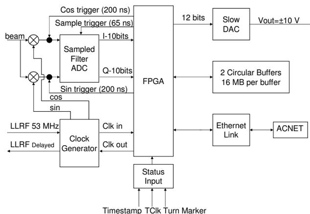
Figure 1: Schematic of the longitudinal phase monitor.
