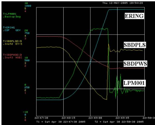
Figure 2: Phase of the first proton bunch (LPM001) from the longitudinal phase monitor, energy (ERING), longitudinal emittance (SBDPLS), and bunch length (SBDPWS). Datas are taken during the ramp of store #4121.
