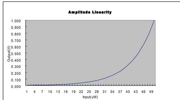
Figure 5: RF signal (350MHz Carrier) amplitude linearity of the prototype digital BPPM
