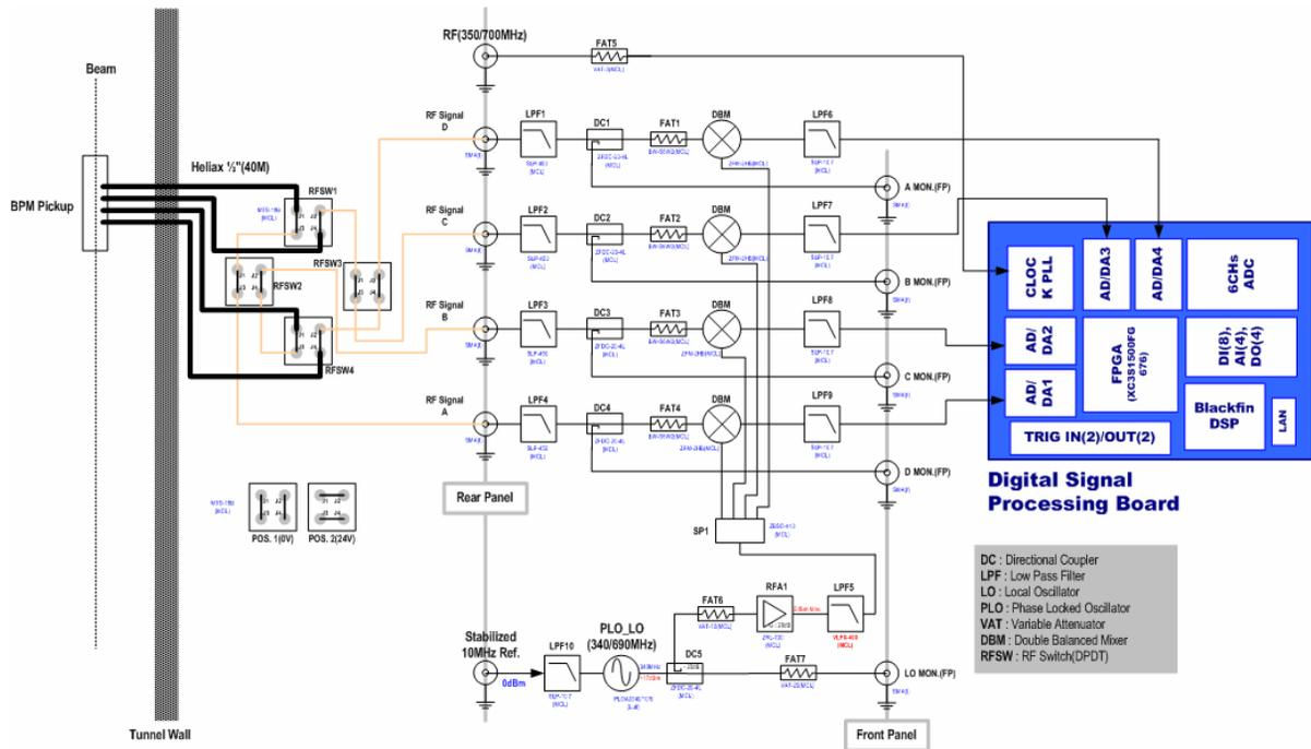
Figure 1: A configuration of the Digital Beam position and Phase Monitoring
