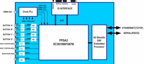
Figure 3: The detailed configuration of the Digital BPPM Core Board
