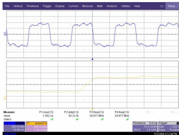
Figure 2: The characteristic of the PLL clock generator
