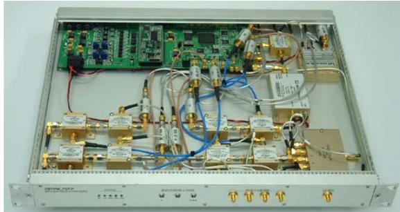
Figure 4: The photograph of the prototype digital BPPM
