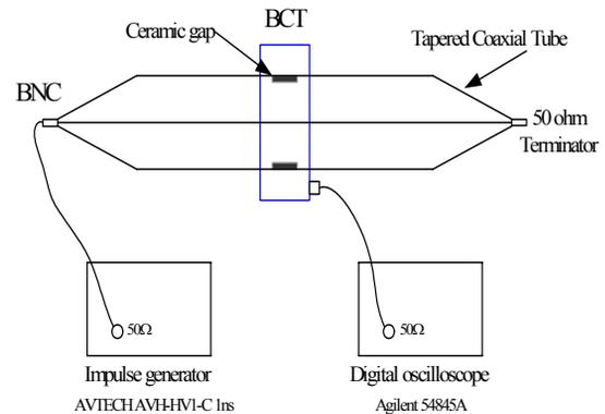
Figure 3: the schematic diagram of BCT calibration.
